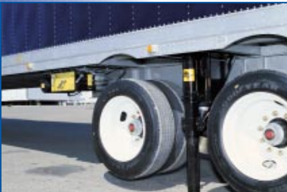
Power Gear® rear mount systems are usually mounted between the rear dual tires on high cube, drop frame trailers. (E-vans)
